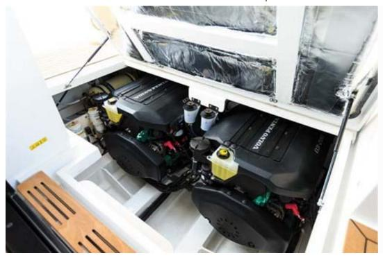
Engine options for the Sealine C330 cruiser are single 330 or 400hp units or twin 170 or 220hp power plants, all Volvo Pentas. Our boat had the most powerful setup: two D3 diesels delivering lively performance and a surefooted Duoprop drive.
