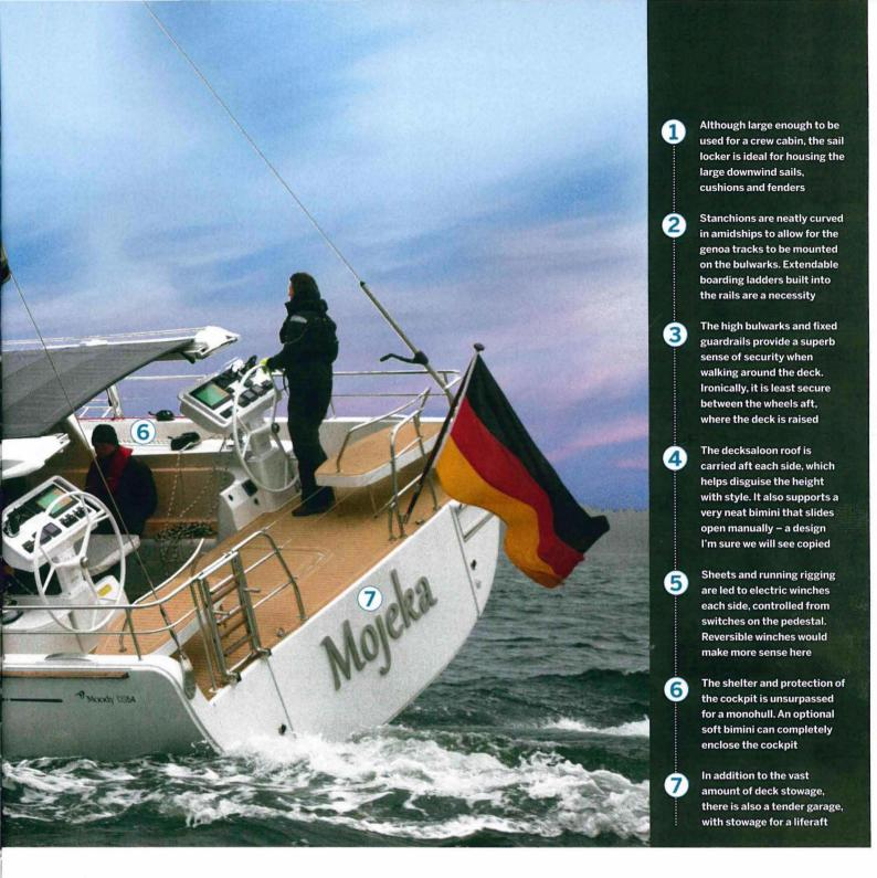
Right: the twinheadsail set-up suits the 54DS perfectly. It allows you to change gear easily from the helm, while keeping full foresails to suit all conditions
