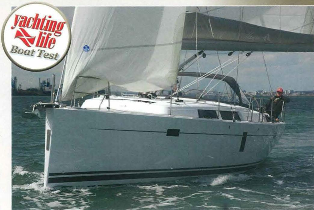
from Selden. Standard mainsail is fully battened with single line slab reefing and lazyjacks working to provide a nice balance with the 106% self tacking blade jib.
