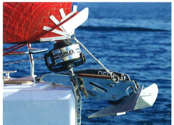
▲ Above: the roller provides stem clearance for the anchor. It has an eye near the forward end to attach the tack of an asymmetric, keeping it clear of the furler
