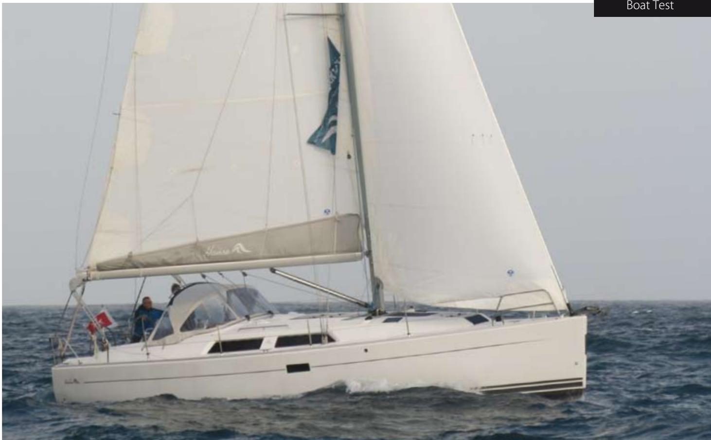
portant ropes lead down the cockpit to the helm, and as with all other Hanse models, her jib is self-tacking. There's also a fully battened North mainsail. She's fast and can cruise at around seven to eight knots given the right conditions - something you appreciate when you learn that an extra knot saves about an hour in a trip to Sicily. The new Hanse 400 also benefits from the novel T-keel, which helps it run at a good clip and reach higher speeds when running on a beam reach.
