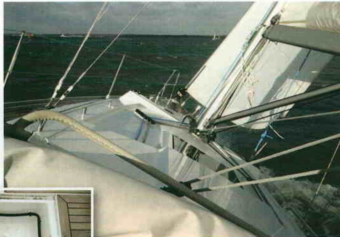
ABOVE Lewmar's flush-fitting hatches were designed into the coachroof, where lines run aft from the mast in troughs. Some more non-slip would be a useful addition. Note the plinth for the self-tacking jib track. LEFT To reach the steering linkage you simply lift a section of the cockpit sole
