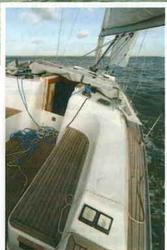
Having the mainsheet on the coachroof makes it hard to control from the wheel, but a traveller in the cockpit is an option. As standard, instruments are mounted on the aft end of the coamings
