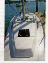
Price as tested: \$186,790 Hull type: Monohull Material: GRP hand laid, polyester resin Length overall: 9.63m Beam: 3.30m Draft: 0.175m (standard); 1.43m (optional) Mainsail area: 28.47m<sup>2</sup> Rec. max. HP: 30 Fuel: 110lt Water: 260lt
