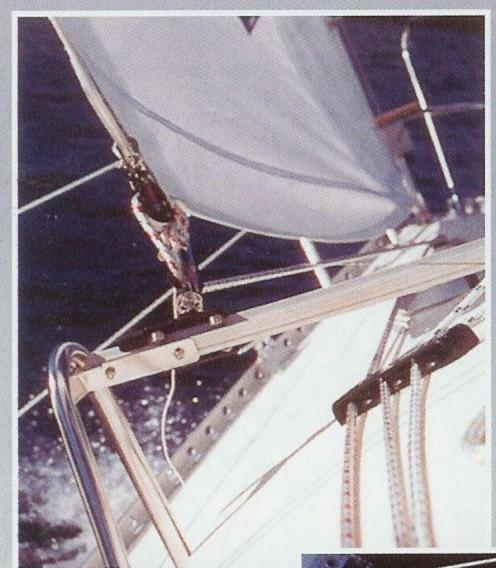
The 301's deck layout is well thought out and makes the boat unusually easy to handle. The selftacking headsail takes all the effort out of short tacking, even in strong winds, and a single-line mainsail reefing system enables one person to reef from the cockpit.
