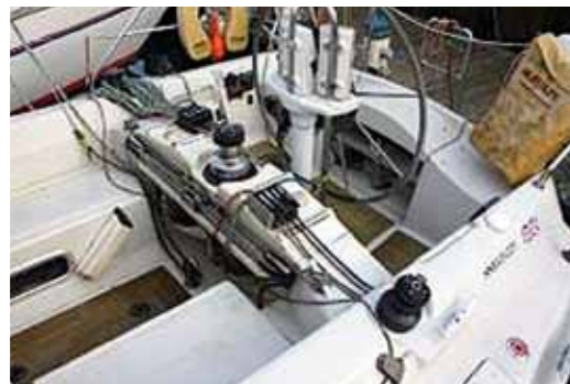
ABOVE The Central Winch System, as introduced on the Dehler 36 CWS
