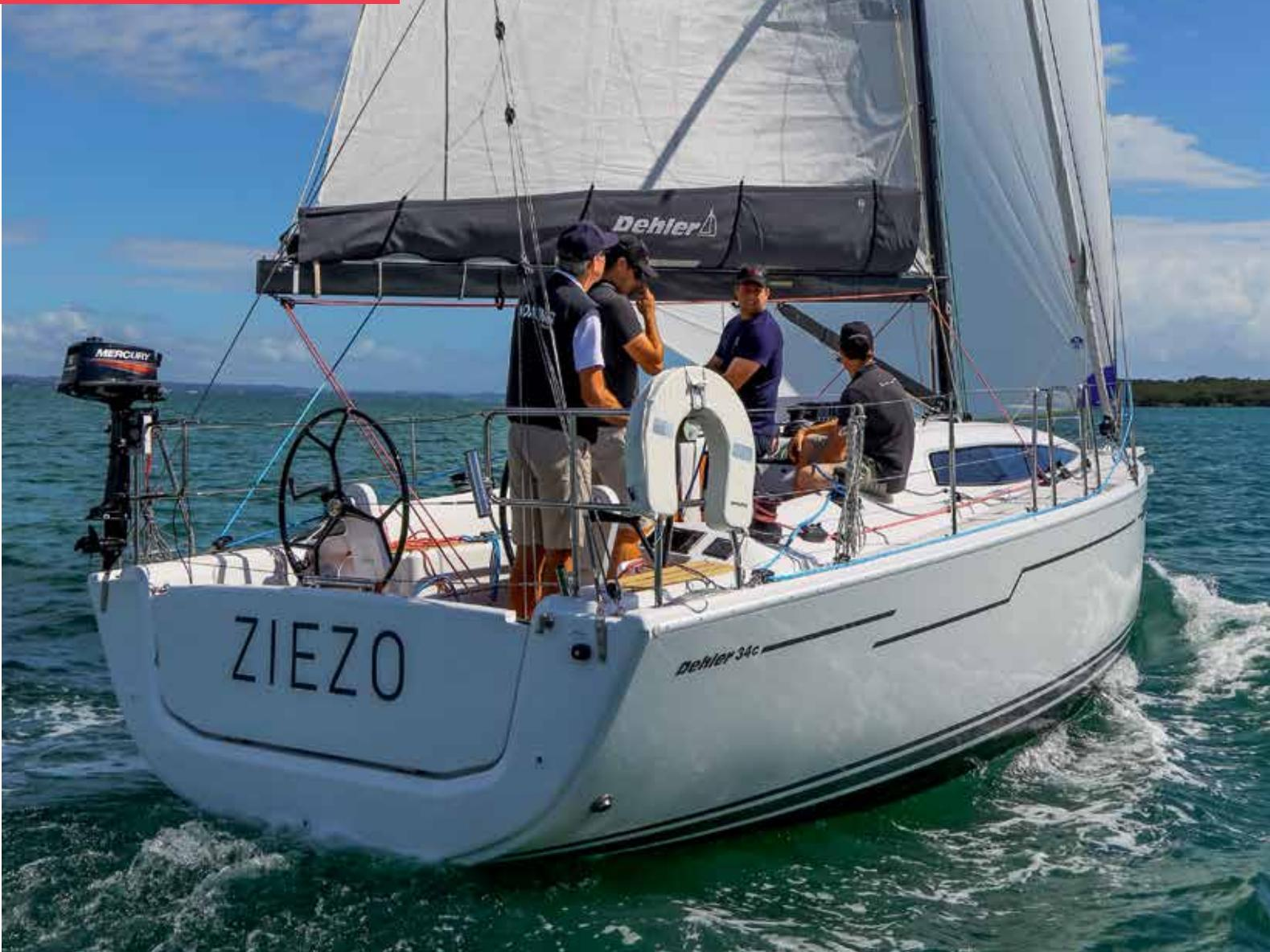
I only have one quibble about the 34's cockpit/rig. The mast has a single backstay that splits about four metres above the helmsman. The starboard split is fitted with a simple but effective block-and-tackle system for encouraging mast bend, but it's irritatingly close to your head/shoulder – even with my average height. I understand the termination point can be shifted to a pad-eye further outboard, which should help.
